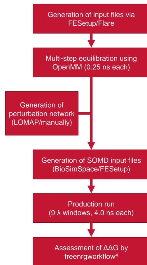
**Figure 4:** Preliminary automated workflow.
